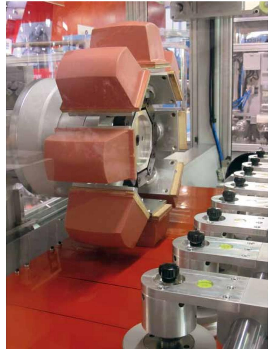
with an interchangeable plate for cliché support where it is possible to mix with high freedom large and small clichés (and large and small ink cups).
