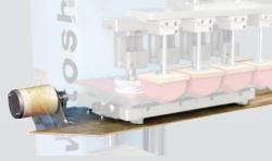
They permit the pads cleaning cycle with programmable operating time.
