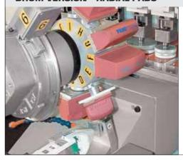
On this configuration pads are disposed radially up to 12 on a drum, to print on differently angled object surfaces.
