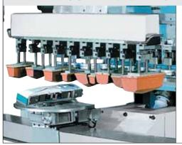
All the pads are aligned on one bar. On this configuration is possible to use as parts conveying accessory either an Indexer (single fixture) or a Rectilinear conveyor (multiple fixtures). With indexer running it is possible to position additional controlled axes to make easier the graphic disposal in one sole cycle even on different sides of the object.
